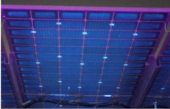
Fig. 4: UVF image from the rear side of a PERC panel showing oxygen diffusing inward from the perimeter. Panels installed in 2018.
